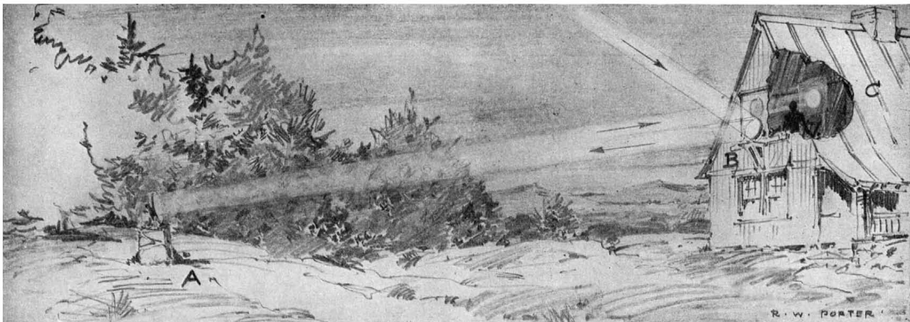
ON THE SPRUCE-CLAD SUMMIT OF BREEZY MOUNTAIN THE VERMONT ASTRONOMERS HAVE BUILT THEIR STELLAR FANE. A SEVENTY-FIVE FOOT SOLAR TELESCOPE PROJECTS THE SUN'S IMAGE ON A SCREEN INDOORS
